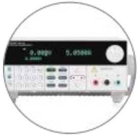
DC voltage regulator/ electronic load
