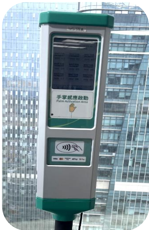
Parking fee collection equipment
