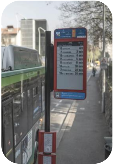
Electronic bus stop sign
