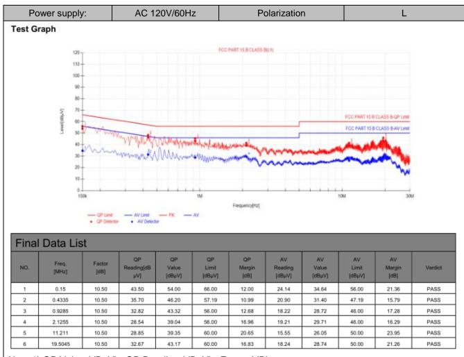
Note:1).QP Value ( $dB\mu V$ )= QP Reading ( $dB\mu V$ )+ Factor (dB)
