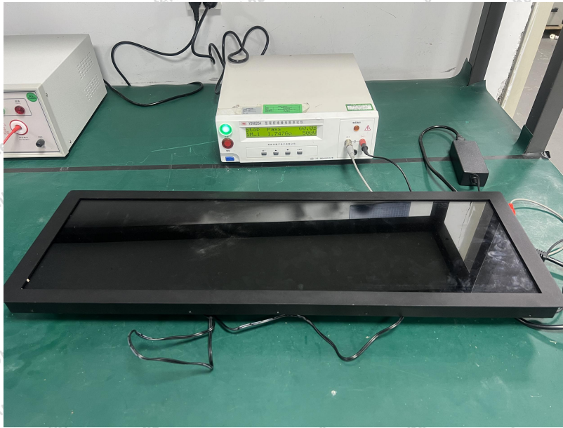
Insulation resistance test - before withstand voltage test
