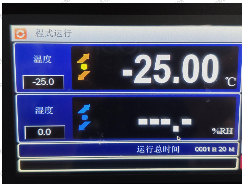
Low temperature start-up test
